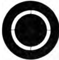
FIG. 163.—Diaphragm showing annulus, the breadth of which may be varied to suit the state of the air.
